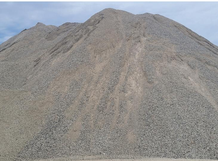
50mm Crushed Concrete
