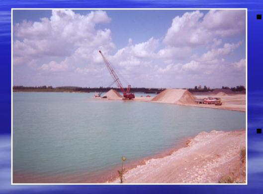
Dredging creates a temporary drawdown effect - imagine taking a handful of sand out of a bucket of sand & water **Groundwater flows** into the pit to offset extraction, resulting in lower water table levels
